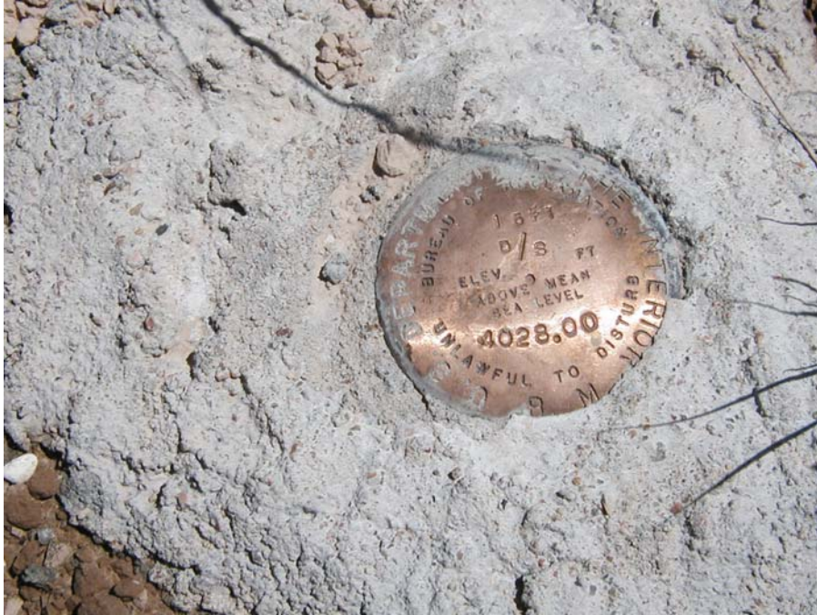
Figure 2 – BOR cap, left abutment, d/s 15-feet, elevation 4028.00.
